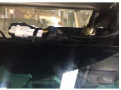
6. Pull knob to turn on the wiper. and press to turn off this will set the wiper blade in the correct position.
