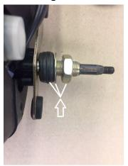
2. Install wiper motor into wiper housing to hold the motor in place. Add the grommet, wash and nut.
