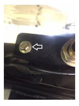
4. Use open end wrench to line the nut up with the bolt. Then tighten all nuts and bolts.
