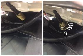
3. Snug passenger side bolt into cage nut on the wiper motor do not tighten at this time.
